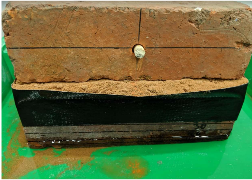
Fig. 29 – Brick on Sand test.
