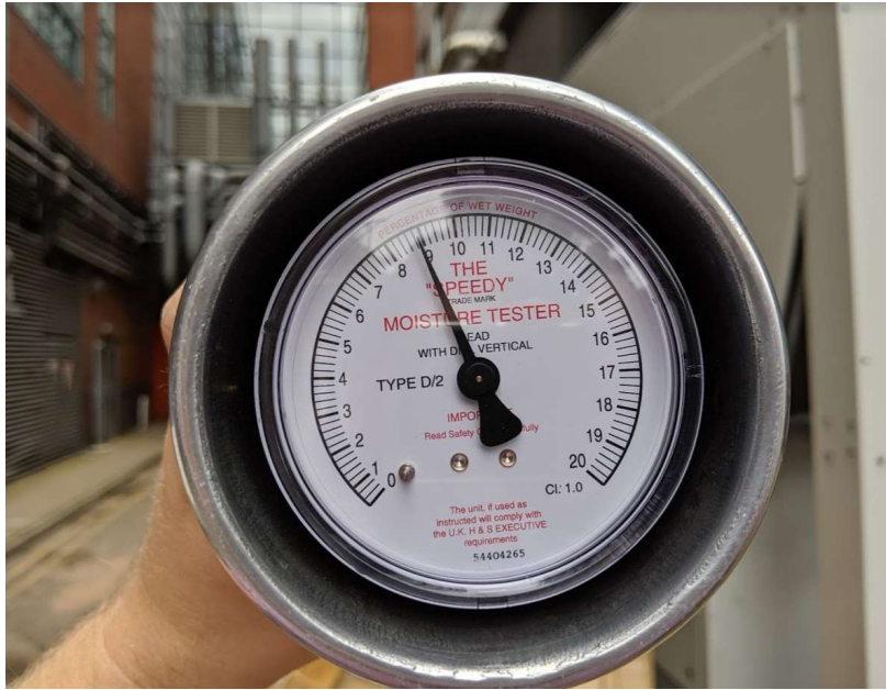
Fig. 60 – Carbide Test – Submersion.
